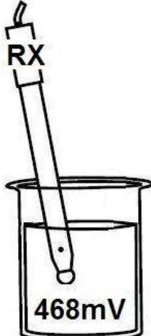
Keep pressing Enter button for 3 seconds to enter in the main Menu. Move the cursor to Calibration and press Enter to do the Calibration.
